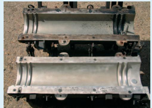
An Aluminium rotational mould before & after cleaning.
