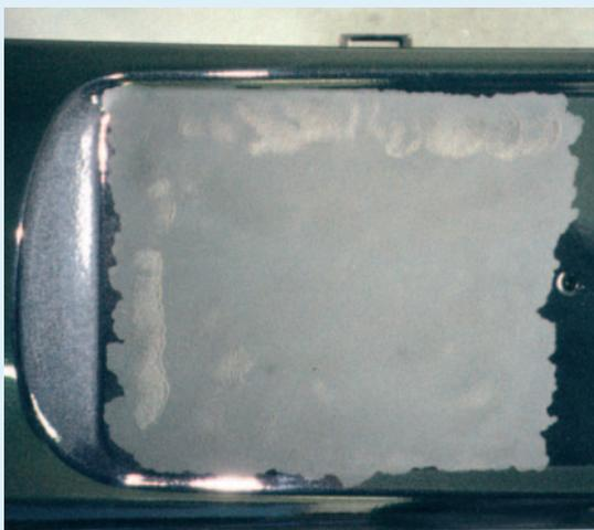
Spalling of automotive bumper during paint removal.
