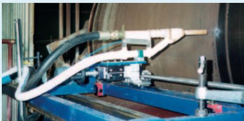
Removing chipboard glue off an endless steel band
