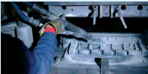
Gravity aluminium die coating removal at 300°C
