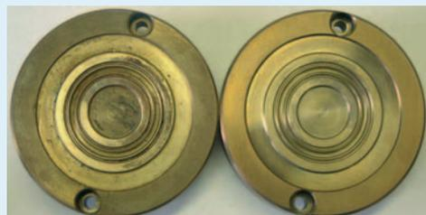
Rubber O-ring mould before & after cleaning
